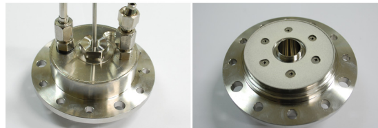
Fig. 4 Fabricated Mixing Head
