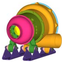
Fig. 6 Finite element model of Turbo Blower
