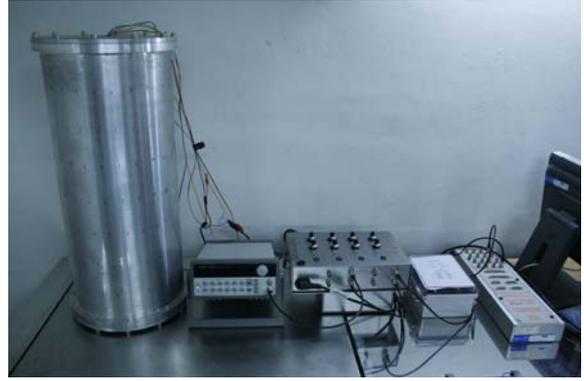
Fig 4. Experimental setup for active vibration control of the stiffened cylindrical shell
