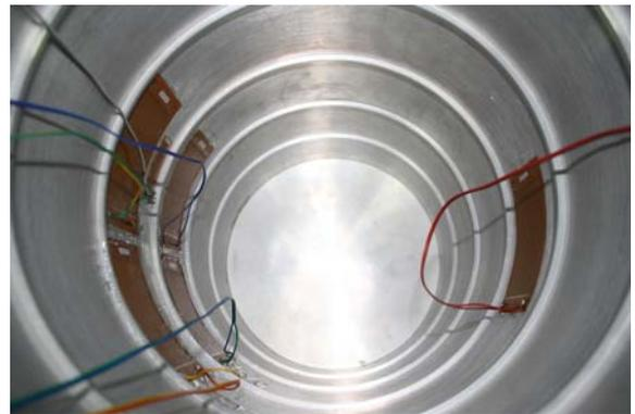
Fig1. Macro-composite Actuators attached to reinforce the Cylindrical Shell
