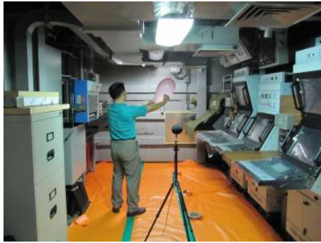
Fig. 2 Impact sound by bursting balloon in a navel vessel
