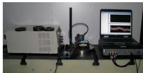
Fig. 1 Apparatus for Friction Plate Run-out Test
