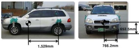
Fig. 1 C.G. of SUV Vehicle
