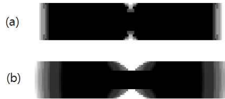
Fig. 1 Optimization result : (a) Frequency Maximization (b) Target Frequency
