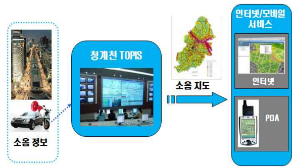
Fig. 3. The web publication process of the noise map
