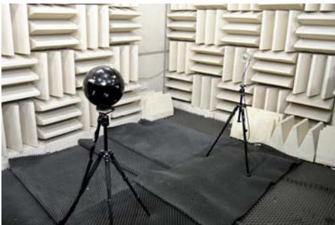
**Fig 1 Experiment Apparatus of Spherical Microphone Array**
