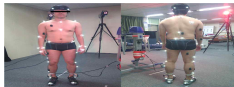
Fig. 2 Infrared reflect marker and wireless EMG sensors
