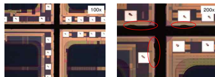
Fig. 2 Chipping image at chip edge after sawing Process
