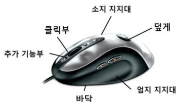
Fig. 1 Configuration view of computer mouse
