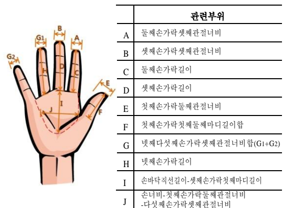
Fig. 2 Size of hand parts relevant to computer mouse
