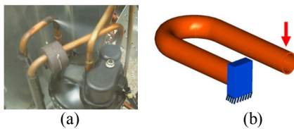
Fig. 1 (a)Failure example and (b)boundary condition
