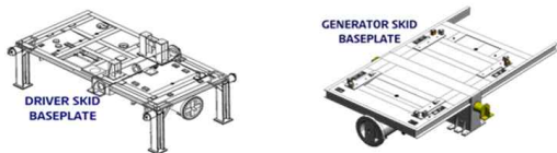
Fig. 1 Baseplate for gas turbine generator package
