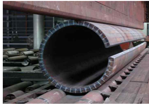
Fig. 3 Press bending process for tube forming
