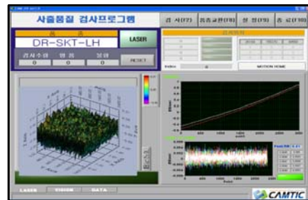
Fig.7 Main frame of inspection program
