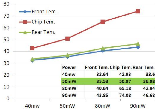
Fig. 5 Thermal analysis by various output power
