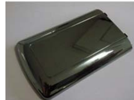
Fig. 5 Image of cellular phone cover using IMD injection molding process
