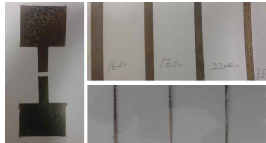
Fig. 2 Spray patterning results through mask
