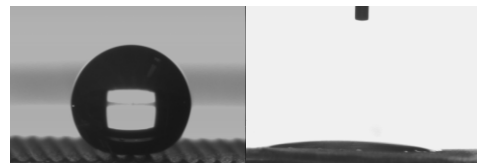
Fig. 3 Contact angle of Micro patterned and non patterned surface
