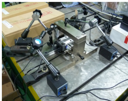
Fig. 2 Experimental setup for measurement of stiffness
