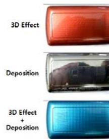
Fig. 5 Result of successful in-mold decoration part for three kinds of thin-film
