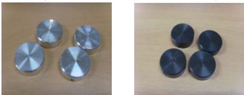
(a) aluminum alloy (b)anodizing
