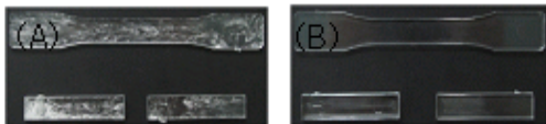
Fig. 3 Appearance of the injection molded specimen using non-dried PMMA with conventional process and new process. (a) Conventional process, (b) pre-pressurized cavity process
