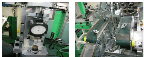
Fig. 6 Depth measurement gauge and Un-loading system
