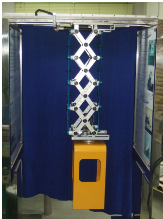
Fig. 3 The test-bed of the vertical moving device using a double scissor mechanism
