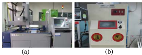
Fig. 1 Equipments for machining turbine blade cooling holes : (a) EMD super drilling machine (b) Shot blast machine
