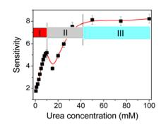
Fig. 2 Sensitivity of sensor showing influence of urea concentration on enzyme activity of cellulose-SnO<sub>2</sub> hybrid nanocomposite urea biosensor
