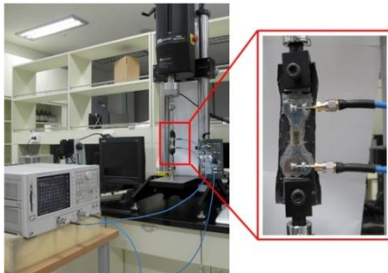
Fig. 3 Frequency measurement for Tire deformation
