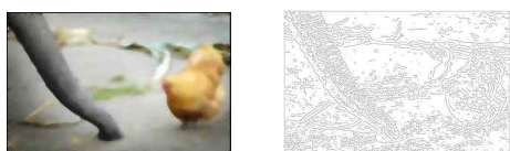
Fig.5 The median filter effect and The Canny effect
