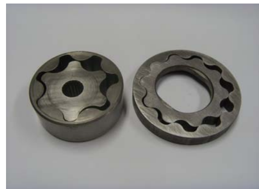
Fig. 12 Samples manufactured by EDM
