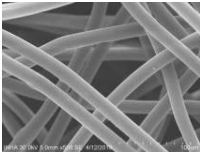
Fig. 2 Surface morphology of Tencel nonwoven (SEM)
