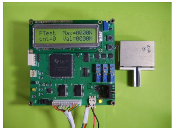
Fig. 2 Manufactured force measuring system of two-finger grasping by three-axis force sensor.
