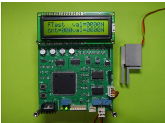
Fig. 1 Manufactured force measuring system of two-finger grasping with one-axis force sensor
