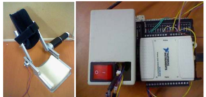
Fig. 2 Developed Exoskeleton Rehabilitation Device and Control Part
