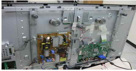
Fig. 4. Two Channel Magnetostrictive Speaker applied in Flat Panel Display
