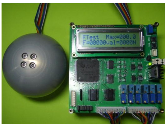
Fig. 5 Manufactured finger-force measuring system
