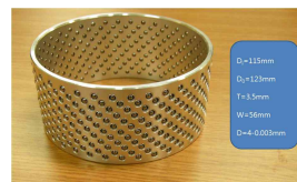
Fig. 2 Photograph of ball bush
