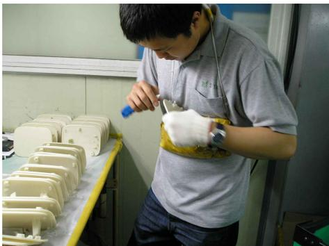
Fig. 1 Image of manual de-burring work using ceramic knife
