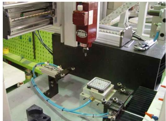
Fig. 3 De-burring system using Orthogonal Robot
