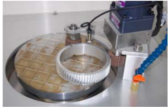
Fig. 1 Mechano Chemical Polishing Machine for sapphire wafer
