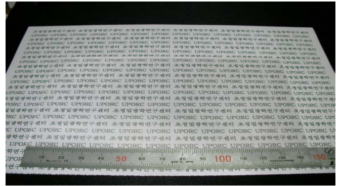
Fig. 5 Lenticular Lens Array without Cross-Talk
