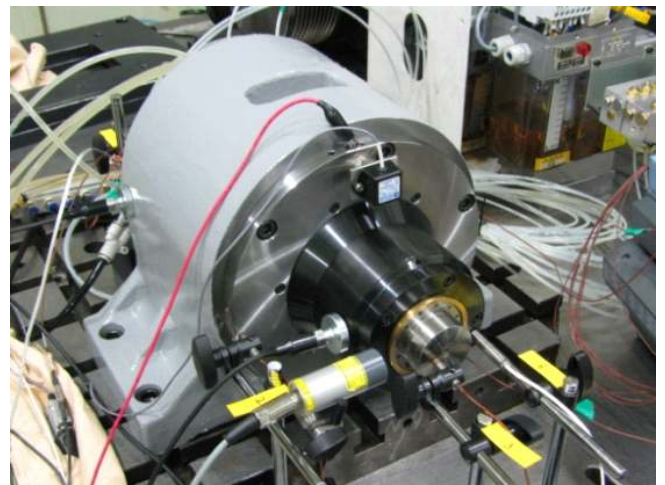
Fig. 2 Experimental Set-up of High Speed Spindle with 40,000 rpm
