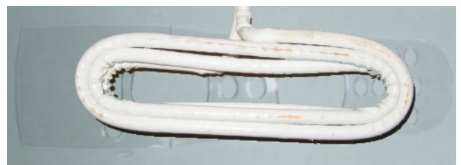
Fig. 3 An elliptic coil designed for induction heating
