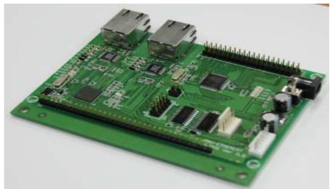
Fig. 3. Picture of EtherCAT slave module
