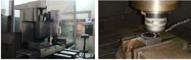
Fig. 5 Generation of gear profile by machining
