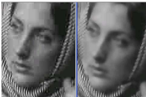
Figure 2 : Comparison of visual quality on Barbara image (0.4 bpp) a) JPEG compressed image (left) b) processed with our method (right)
