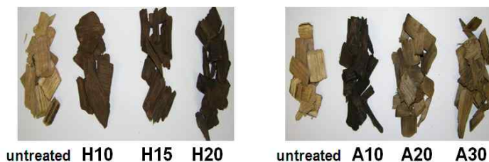
Fig. 1. Hot water and alkali pre-extracted chips as a different pre-extraction yield.
