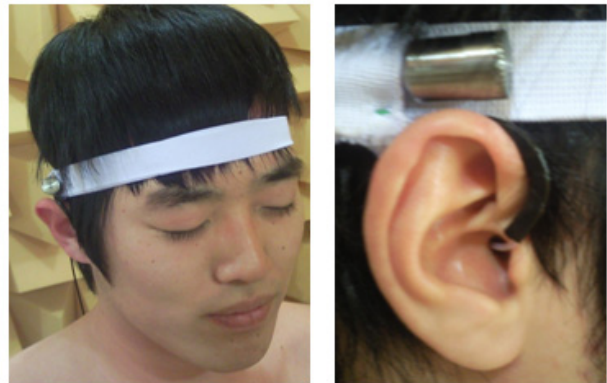
Fig.1 Experiment set-up (set-up of probe and reference microphone)
