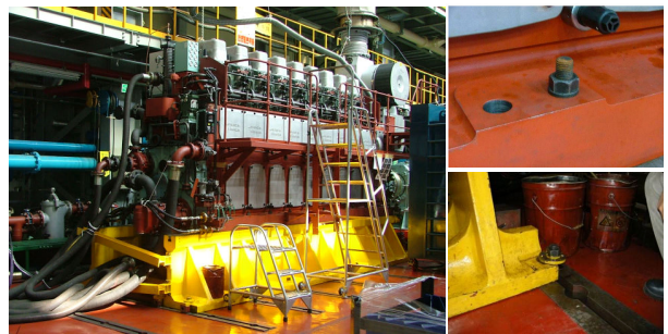
Fig. 2 Installation condition of engine(test shop)
