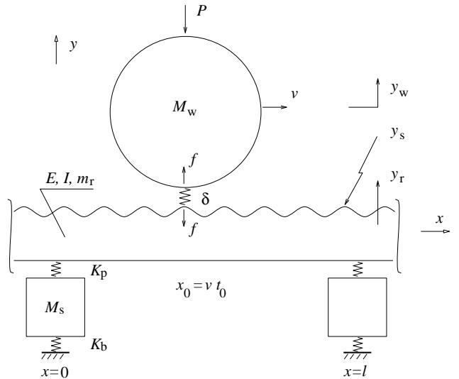
The vertical rail deflection,  $y_r(x_0, t_0)$ , at the moving point,  $x_0 = vt_0$ , (under the wheel) is a convolution of the rail Green's function,  $g(x, x_0; t, t_0)$ , and the contact force  $f(x, t)$ ,
