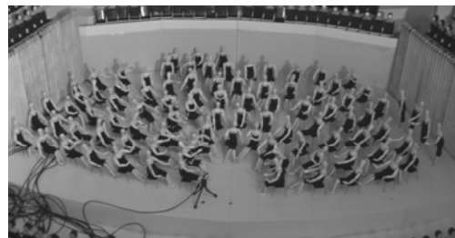
Fig 1 Orchestra player in a 1:10 scale model
