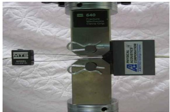
Fig. 1 Transducer location of fatigue crack growth test
